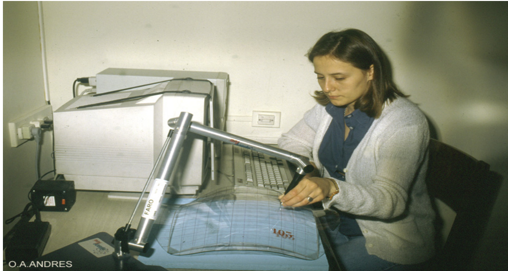
Fig. 9. Scanning the model by the SpaceArm.
