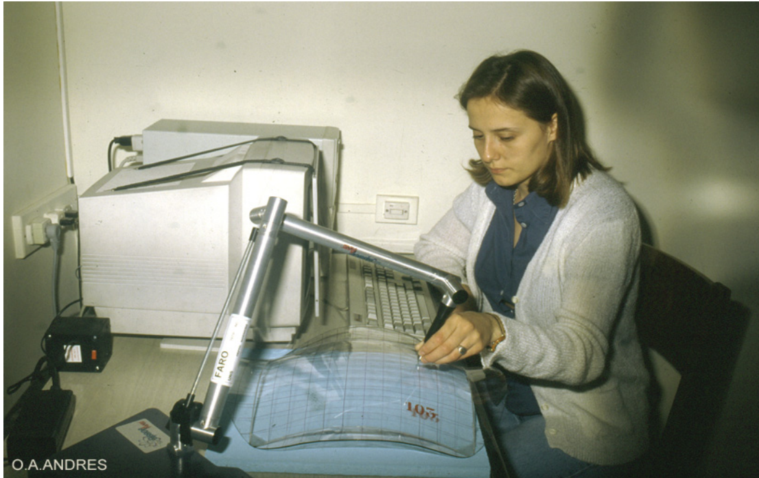
Fig.10. Scanning the model by the SpaceArm.
