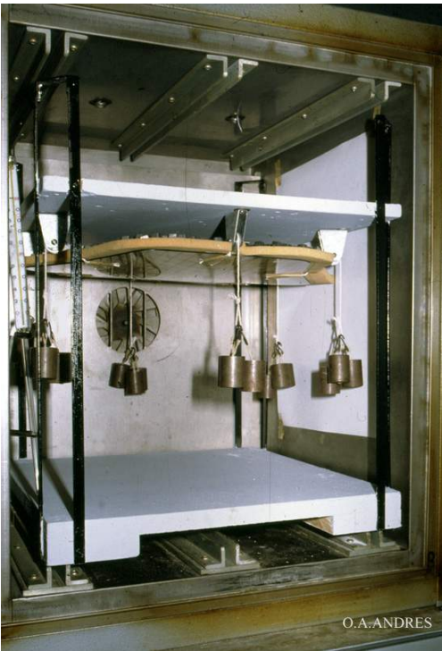
Fig. 2 The mother plate in the oven.
